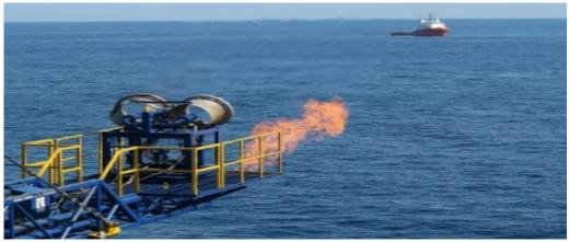
Fig. 3. Flame of methane gas burning during the operation test of methane hydrates made by Japan in the Pacific Ocean
