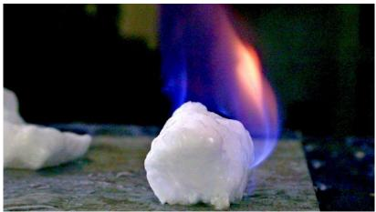
Fig.2. Example of flammable ice
